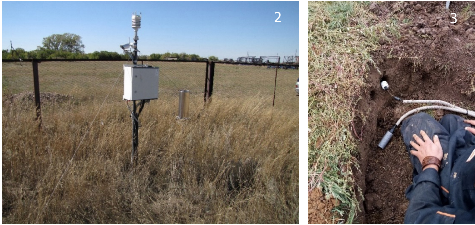
Figures 2–3. 2. Meteorological station in Poluyamki village (photo by Bondarovich). 3. Installation of the "Hydra Probe" (Stevens, USA) of the soil hydrological station (photo by Bondarovich).
