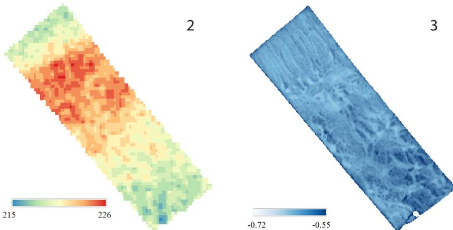
**Figures 2–3.** 2 – Digital model of the relief in field No. 47. 3 – Map of the spatial distribution of the S2WI values in field No. 47.
