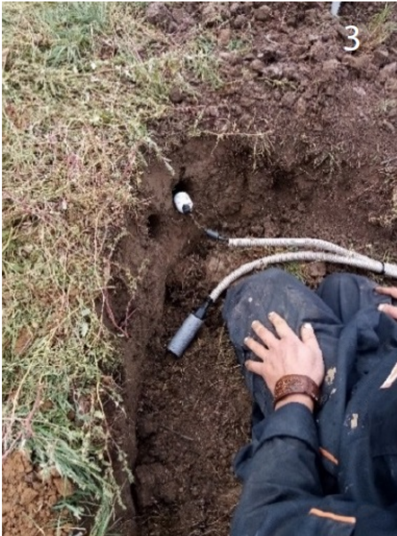
Figure 3. Installation of the "Hydra Probe" (Stevens, USA) of the soil hydrological station (photo by Bondarovich).
