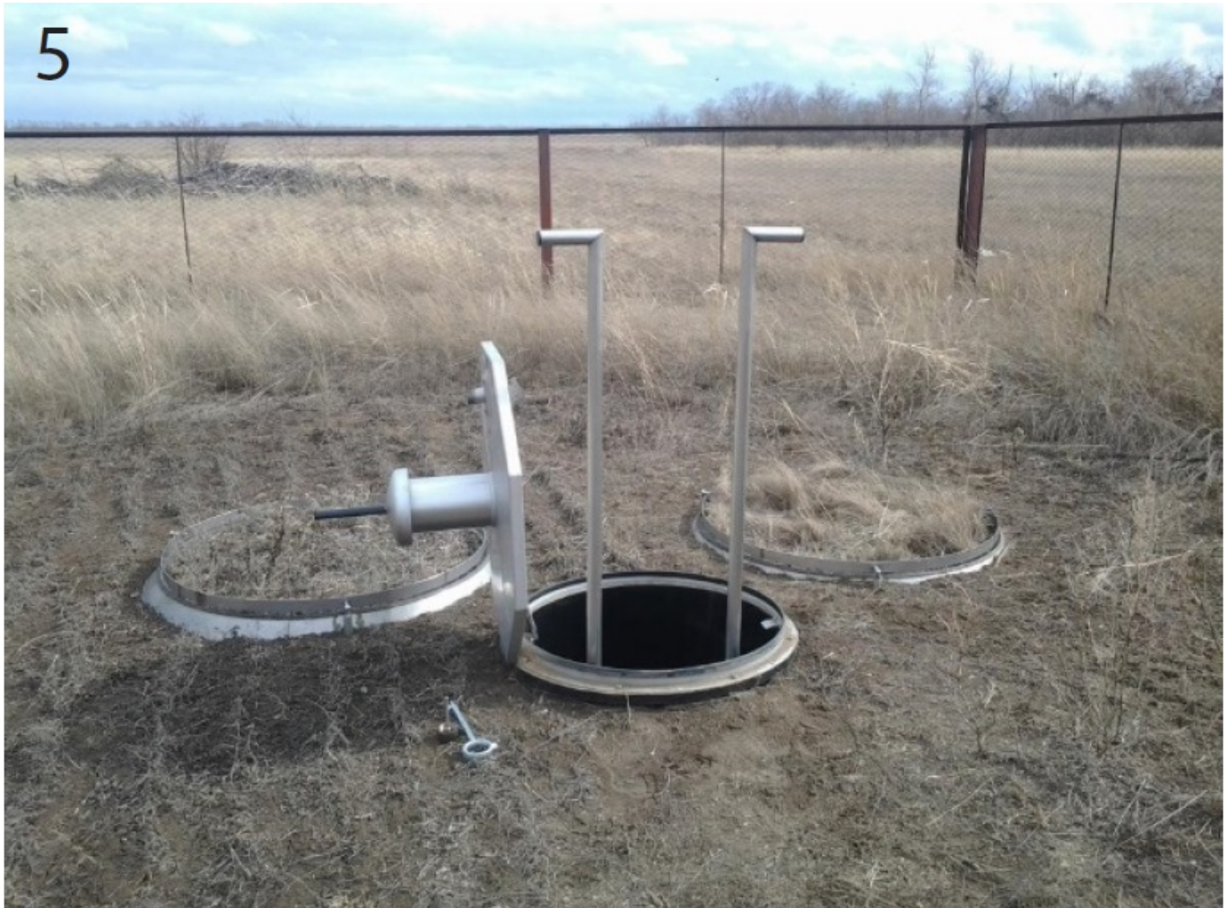
Figure 5. Above-ground part of the two-section (Lys 1 – left section, Lys 2 – right ) gravity lysimeter in the village of Poluyamki (photo by Bondarovich).
