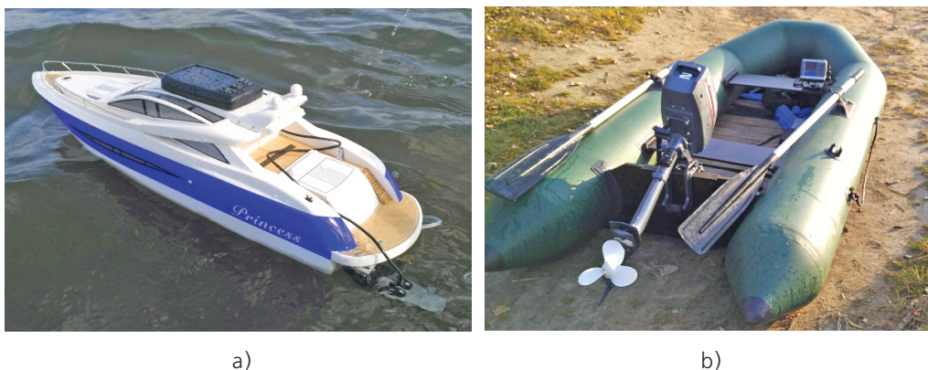
Fig. 5. Bathymetric survey equipment: a) autonomous bathymetric vessel; b) boat with an echo sounder
